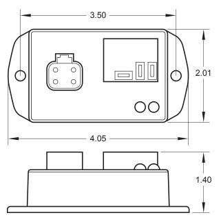
The Innovative Controls Inc. model 3050510-03 High Idle Relay is used to monitor the vehicle battery voltage and energize a relay when a low voltage condition is detected. The relay is typically used to increase the engine idle speed so that the alternator can recover the battery voltage. The High Idle Relay is a fully potted module that is suitable for automotive applications.
